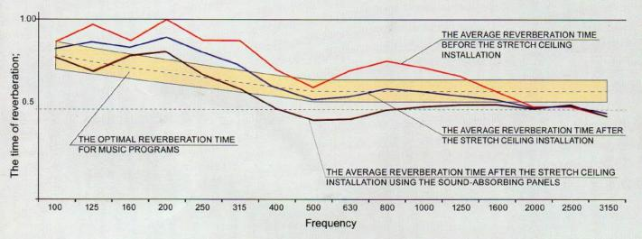
In most cases, it is enough to install SAROS DESIGN COMFORT stretch ceiling for good noise absorption in the room. At the same time, it is advisable to make the height of the ceiling void at least 10 cm.
