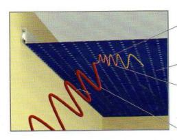
THE TRANSFORMATION OF THE SOUND WAVE ENERGY INTO HEAT ENERGY IN THE HOLES OF STRETCH CEILING
